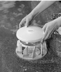
3) Snap Vortex filter top in place
